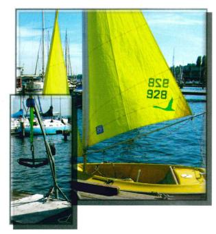
Our fleet of eight sailboats, including Columbia 21s, Access dinghies and Martin 16s, are designed to accommodate a wide range of disabled sailors. We have two boats equipped with electronic controls and a mechanized transfer lift so that anyone can enjoy the freedom of sailing.
